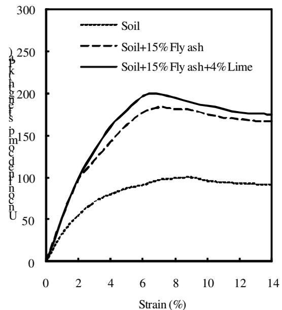
**Fig. 1:** Stress-Strain Behavior of Stabilized Soil at Optimum Content of Fly Ash and Fly ash + Lime
