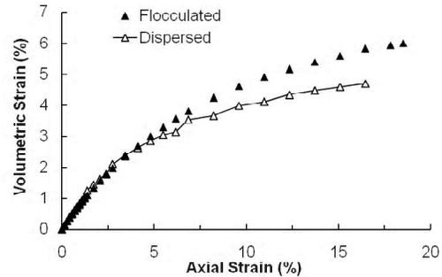
Fig. 5 Variations of Volumetric Strain with Axial Strain of Flocculated and Dispersed Samples Subjected to CD Test Under a Confining Pressure of 200 kPa
