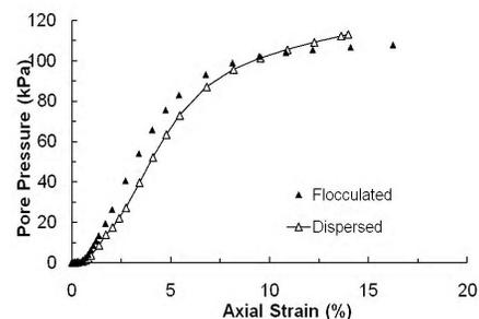
**Fig. 2:** Variations of Pore Pressure with Axial Strain for Flocculated and Dispersed Samples Subjected to CU Test Under a Confining Pressure of 200 kPa
