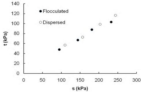
Fig. 3: Modified Failure Envelopes of Flocculated and Dispersed Samples Subjected to CU Test
