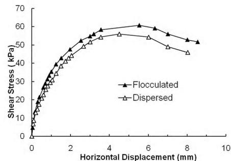
Fig. 7: Variations of Shear Stress with Displacement for Flocculated and Dispersed Samples Subjected to Direct Shear Test Under a Normal Stress of 150 kPa
