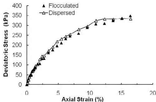
Fig. 4: Stress-Strain Curves of Flocculated and Dispersed Samples in CD Tests Under a Confining Pressure of 200 kPa
