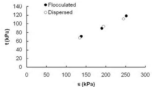
Fig. 6: Modified Failure Envelopes of Flocculated and Dispersed Samples Subjected to CD Test
