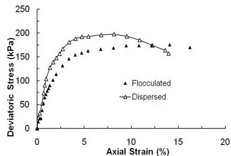
**Fig. 1:** Stress-Strain Graphs of Flocculated and Dispersed Samples Subjected to CU Test Under a Confining Pressure of 200 kPa
