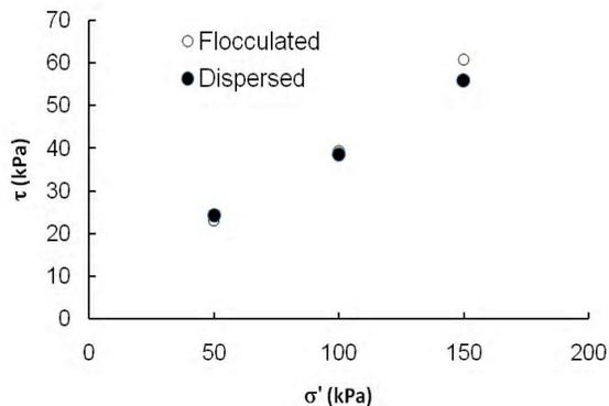
**Fig. 8:** Failure Envelopes of Flocculated and Dispersed Samples Subjected to Direct Shear Test
