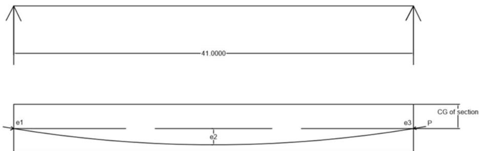
$P = 12000 \text{ KN}$  ,  $e_1 = e_3 = 0$  ,  $e_2 = 1.0 \text{ m}$
