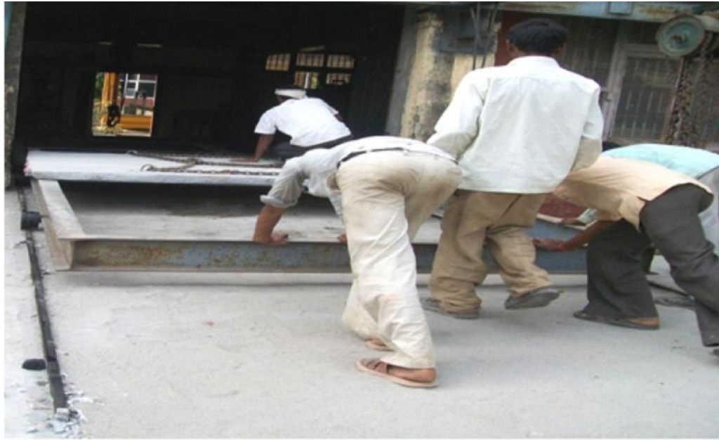
Fig. 3.8: Slab being taken inside the Laboratory
