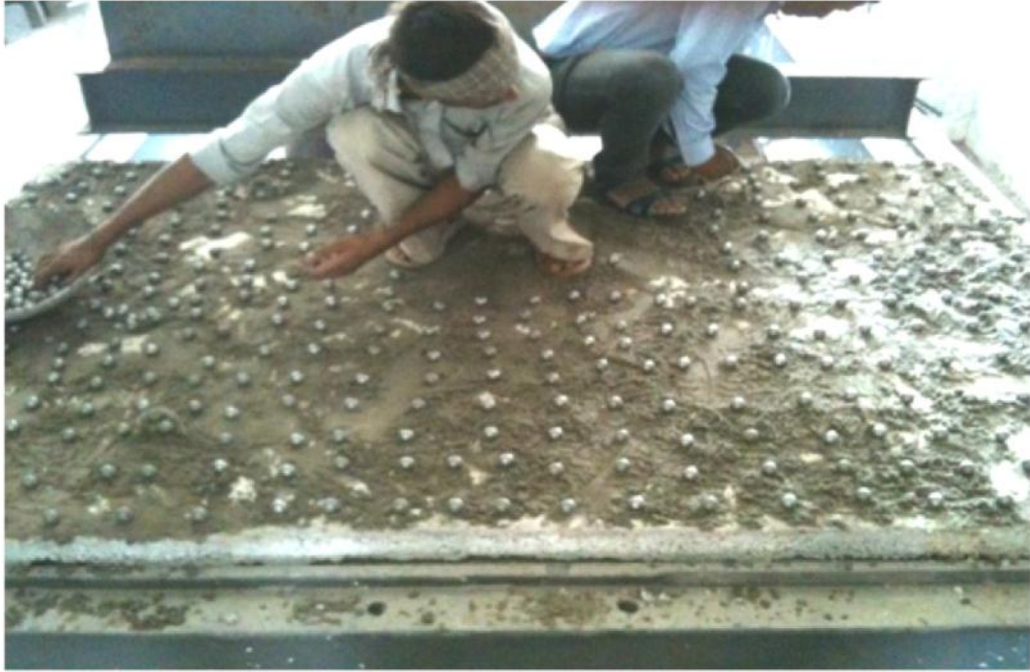
Fig. 3.10: Steel balls used for load conversion
