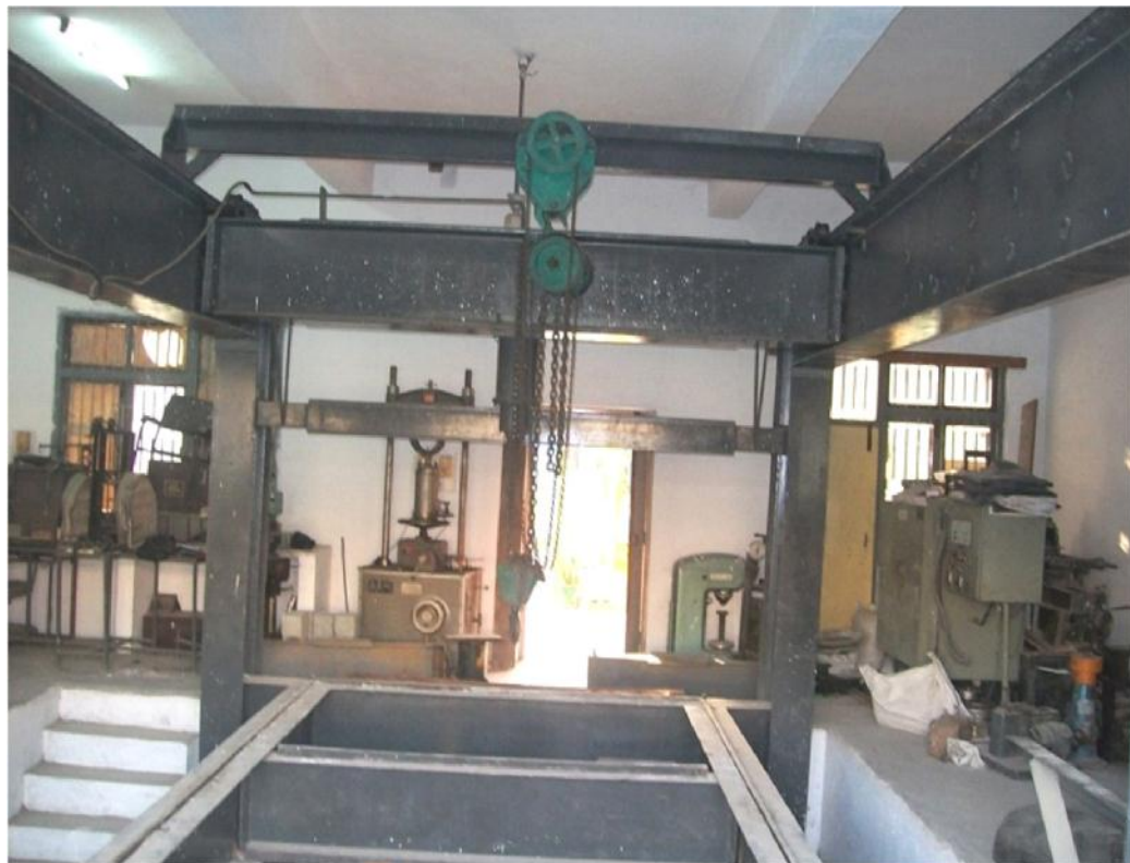
Fig. 3.9: Reaction Frame of Heavy Testing Laboratory
