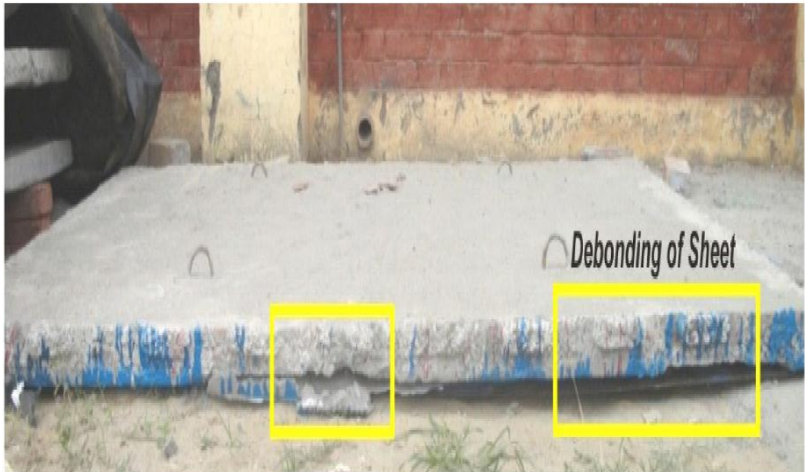
Fig.5.29: Complete Split-up of MS Plate (typical)
