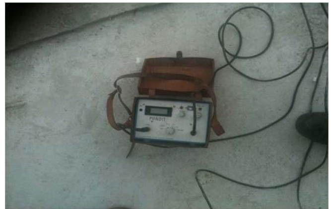
Figure 2. Ultrasonic Pulse Velocity Test machine
