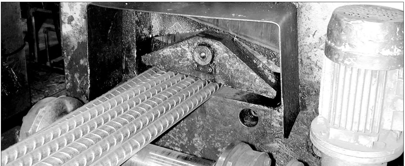
Figure 27: Guillotine shear cutting reinforcement
