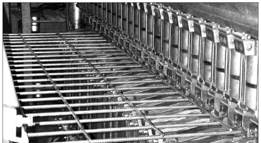
Figure 42: Mesh production by automatic welding machines
