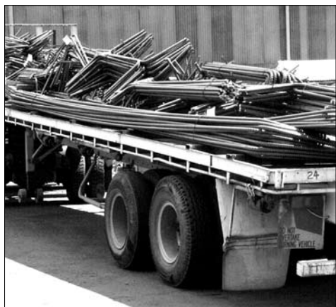
Figure 26: Trailer loaded with reinforcement ready to be delivered to site
