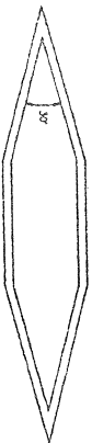
Piers with triangular cut and ease waters, the angle included between the faces being 30 degrees or less
