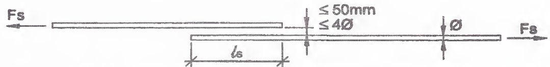
(a) Maximum Spacing Between Two Lapped Bars
