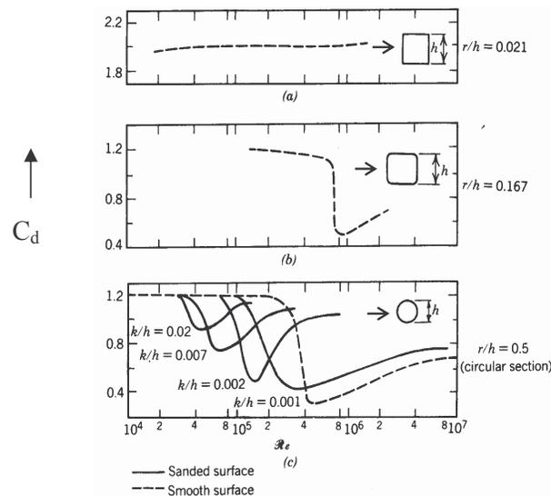
**Figure 8: Influence of Reynolds number, corner radius, and surface roughness on drag coefficient, square to circular cylinders (r is the corner radius; k is the grain size of sand)**
