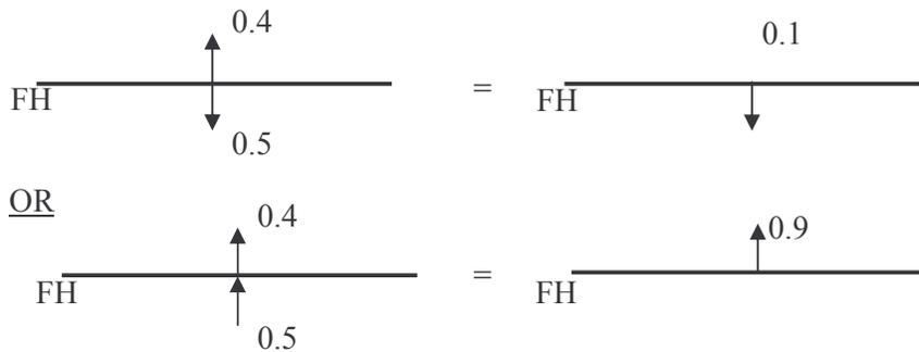
**Figure 1.2- Net Roof Pressure Coefficients for different zones and combinations**
