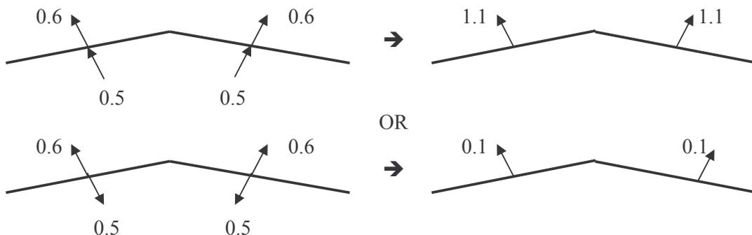
**Figure 6.2 - Net Roof Pressure Coefficients for different zones and combinations**
