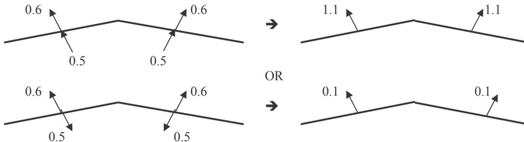
**Figure 4.2- Net Roof Pressure Coefficients for different zones and combinations**
