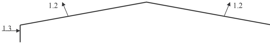
**Both slopes at +ve pressure coefficients and  $\phi = 1$  (case 4)**
