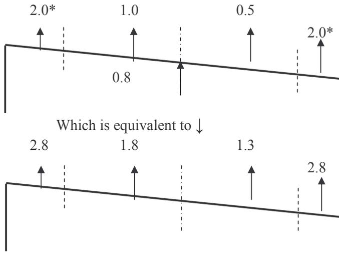
**For  $180^\circ$  wind incidence,  $C_{pi} = -0.4$**
