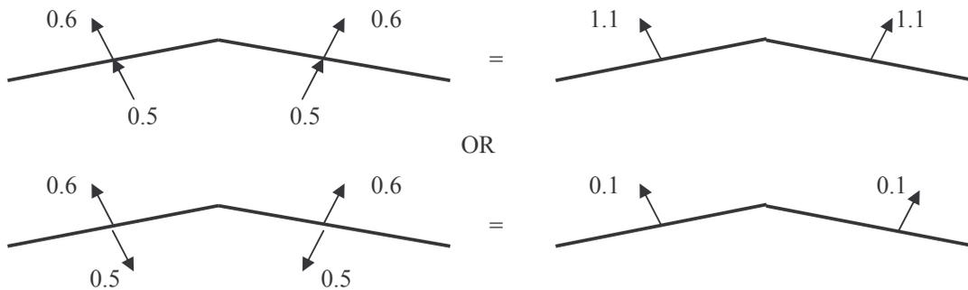
**Figure 14.2 -Net Roof Pressure Coefficients for different zones and combinations**
