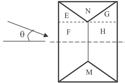
Figure 15.2 - Plan of the building. M,N are hipped slopes
