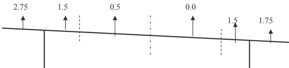
**For 90° wind incidence,  $C_{pi} = +0.5$ , up to  $w/2$  from ends**
