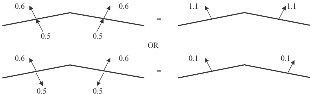
**Figure 13.2 - Net Roof Pressure Coefficients for different zones and combinations**
