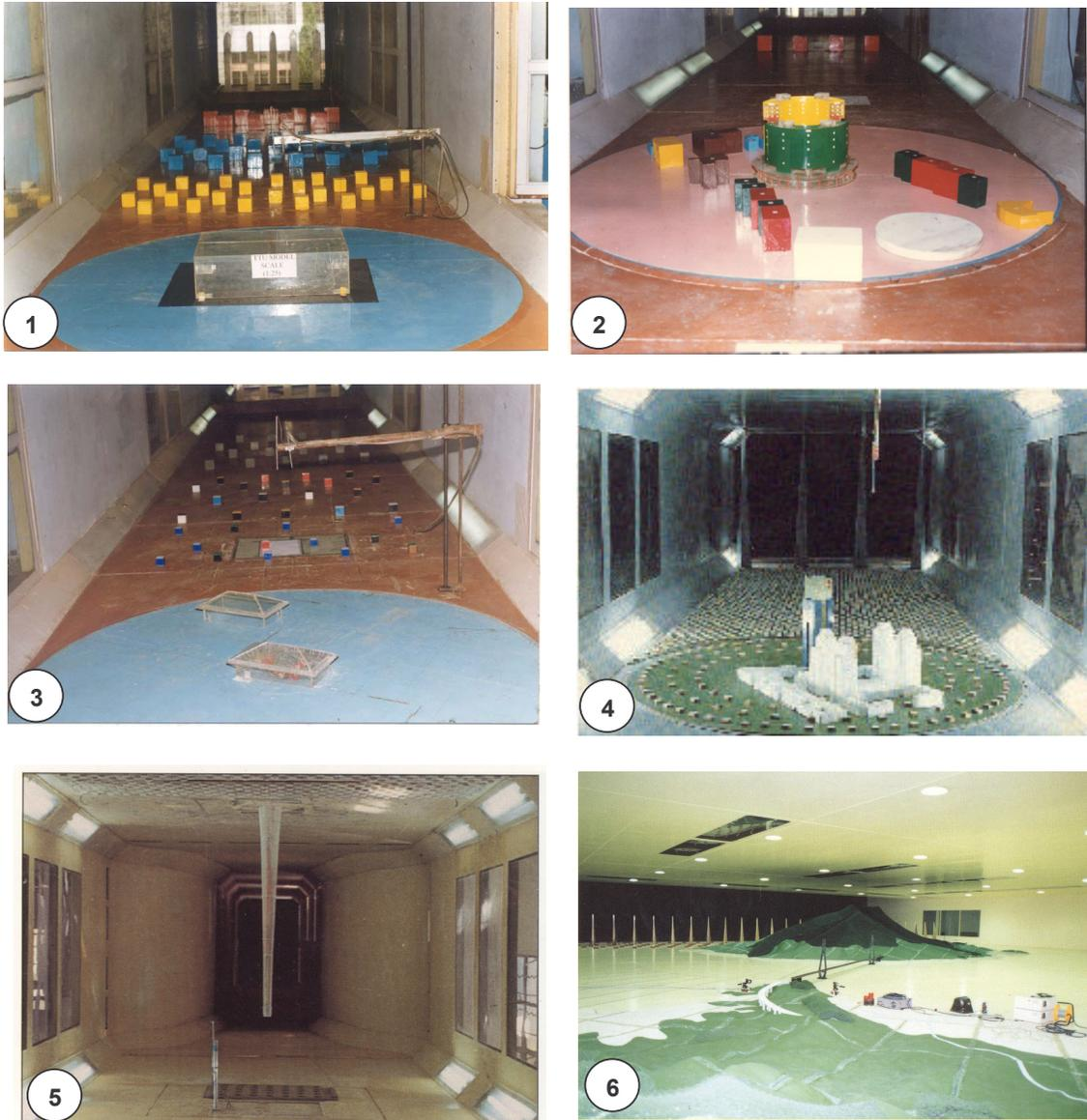
1,2 Building models; 3,4 Study of interference; 5, Chimney model under study; 6, Study of the effect of topography on a bridge model.
