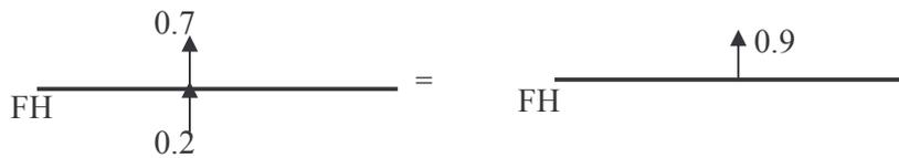
**Figure 3.2- Net Roof Pressure Coefficients for different zones and combinations**
