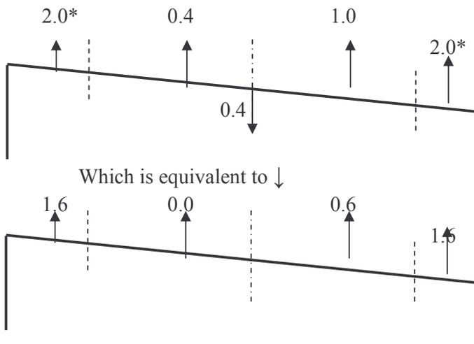
**For  $90^\circ / 270^\circ$  wind incidence,  $C_{pi} = -0.5$ , up to  $w/2$  from ends**
