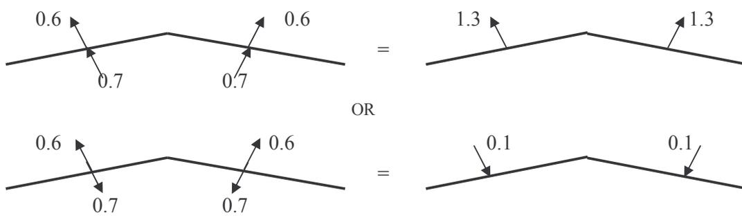
**Figure 7.2 - Net Roof Pressure Coefficients for different zones and combinations**
