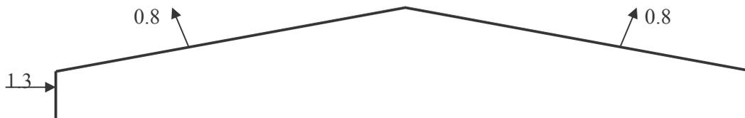
**Both slopes at +ve pressure coefficients and  $\phi = 0$  (case 2)**
