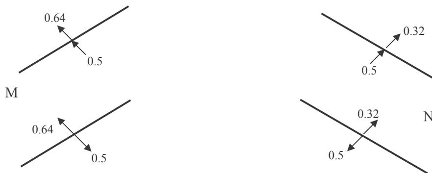
**Figure 15.3- Net Roof Pressure Coefficients for different zones and combinations**
