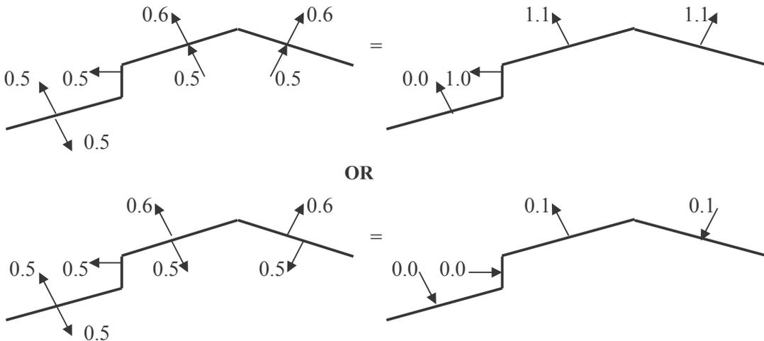
**Figure 11.2 - Net Roof Pressure Coefficients for different zones and combinations**
