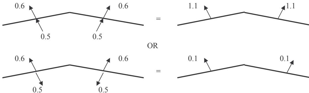
**Figure 12.2 - Net Roof Pressure Coefficients for different zones and combinations**
