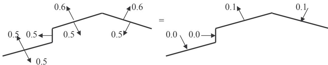
**Figure 10.2 - Net Roof Pressure Coefficients for different zones and combinations**
