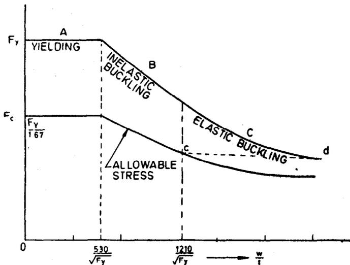
FIG. 15 UNSTIFFENED ELEMENT FAILURE STRESSES AND ALLOWABLE STRESSES FOR  $0 < \frac{w}{t} < 60$
