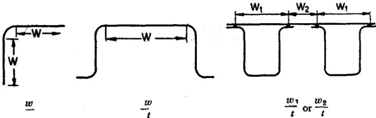
FIG. 6 FLAT WIDTH RATIO
