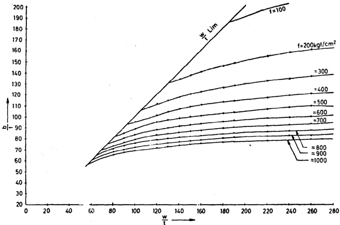
FIG. 26A  $\frac{b}{t}$  RATIO FOR DEFLECTION DETERMINATION (NON-TUBULAR SECTIONS)
