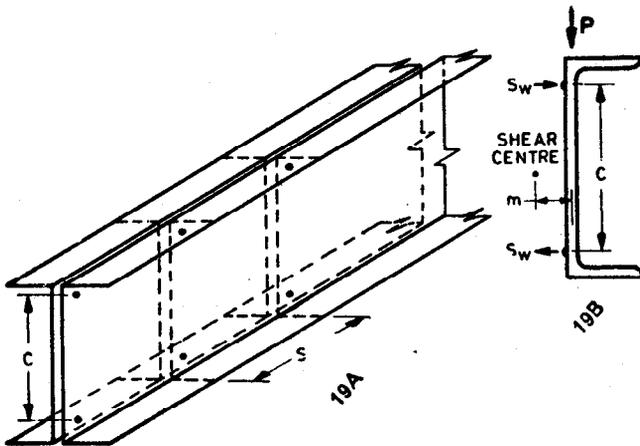
FIG. 19 CHANNELS SPOT WELDED TO FABRICATE I-BEAM
