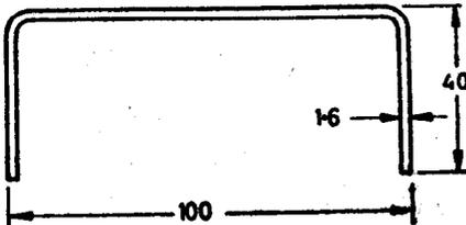
Channel  $100 \times 40 \times 1.6$  ( conforming to Table III of IS : 811-1965 )
