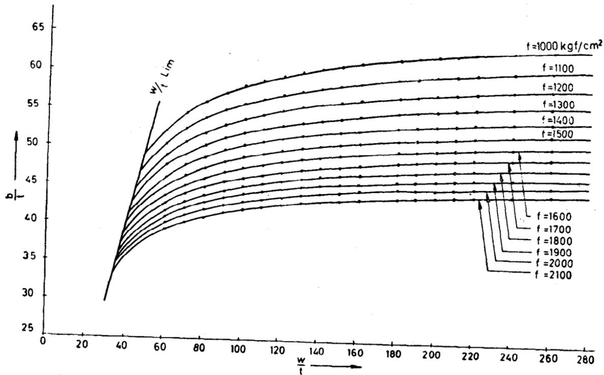
FIG. 27B  $\frac{b}{t}$  RATIO FOR LOAD DETERMINATION ( TUBULAR SECTIONS )
