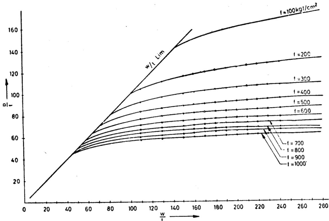
FIG. 25A  $\frac{b}{t}$  RATIO FOR LOAD DETERMINATION (NON-TUBULAR SECTIONS)
