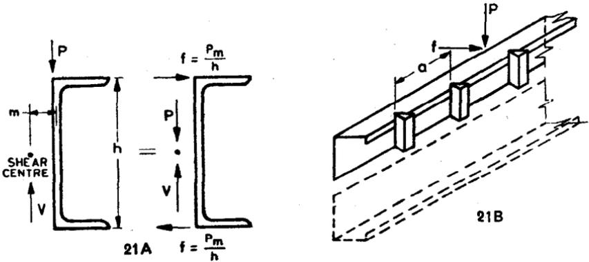
FIG. 21 LOAD ACTING AT THE SHEAR CENTRE — ITS EFFECTS ON THE BRACES
