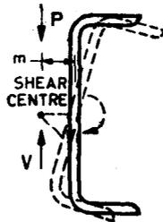
FIG. 18 SHEAR CENTRE OF A CHANNEL
