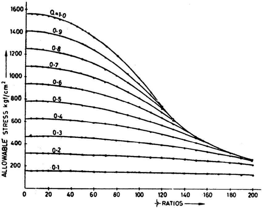
FIG. 35 ALLOWABLE COMPRESSIVE STRESS IN kgf/cm<sup>2</sup>,
