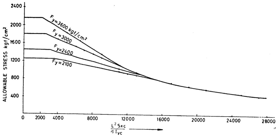
FIG. 30 ALLOWABLE BENDING STRESSES IN kgf/cm<sup>2</sup>, FOR LATERALLY UNBRACED BEAMS
