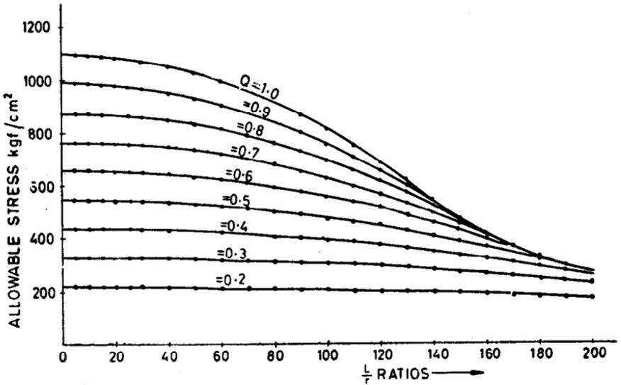
FIG. 33 ALLOWABLE COMPRESSIVE STRESS IN kgf/cm<sup>2</sup>,
