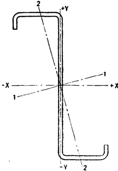
FIG. 22 PRINCIPAL AXES IN Z-SECTIONS
