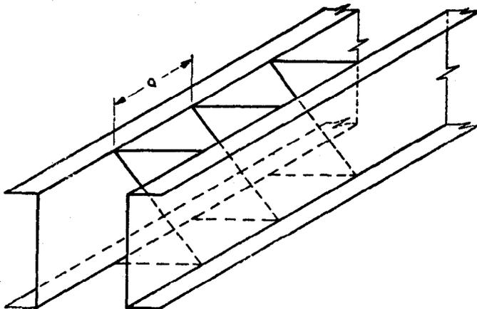
FIG. 20 BRACED CHANNELS
