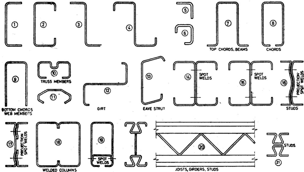
FIG. 1 LIGHT-GAUGE SHAPES FOR STRUCTURAL FRAMING
