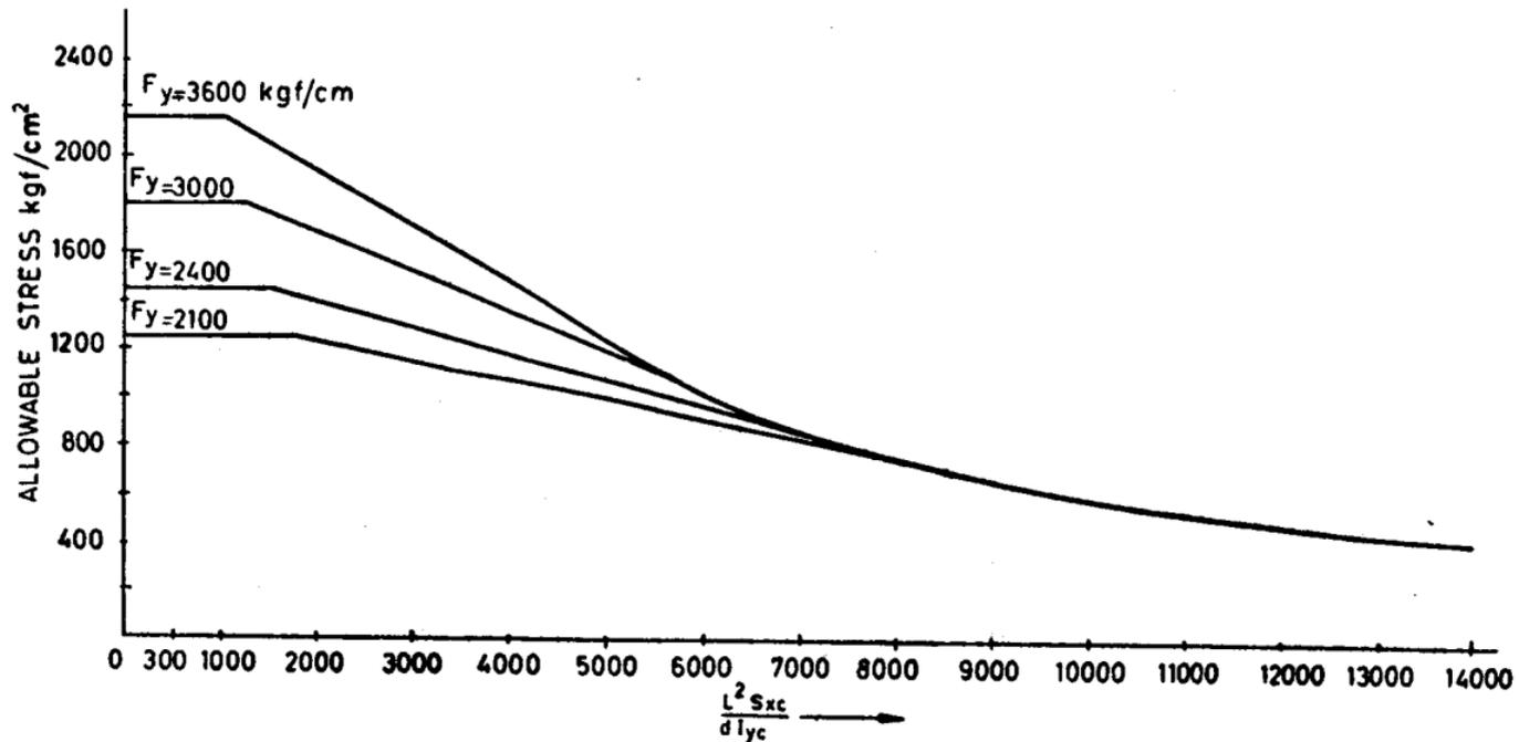
FIG. 31 ALLOWABLE BENDING STRESS IN  $\text{kgf/cm}^2$ , FOR LATERALLY UNBRACED BEAMS (Z-SECTIONS)
