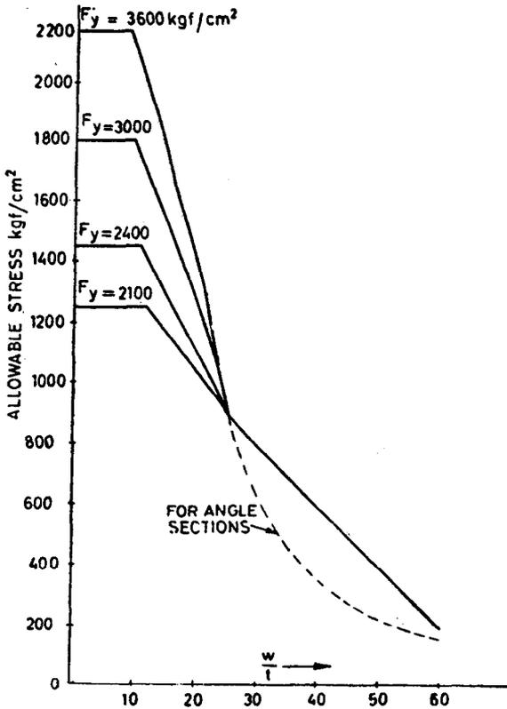
FIG. 29 ALLOWABLE COMPRESSIVE STRESS FOR UNSTIFFENED ELEMENTS, kgf/cm<sup>2</sup>
