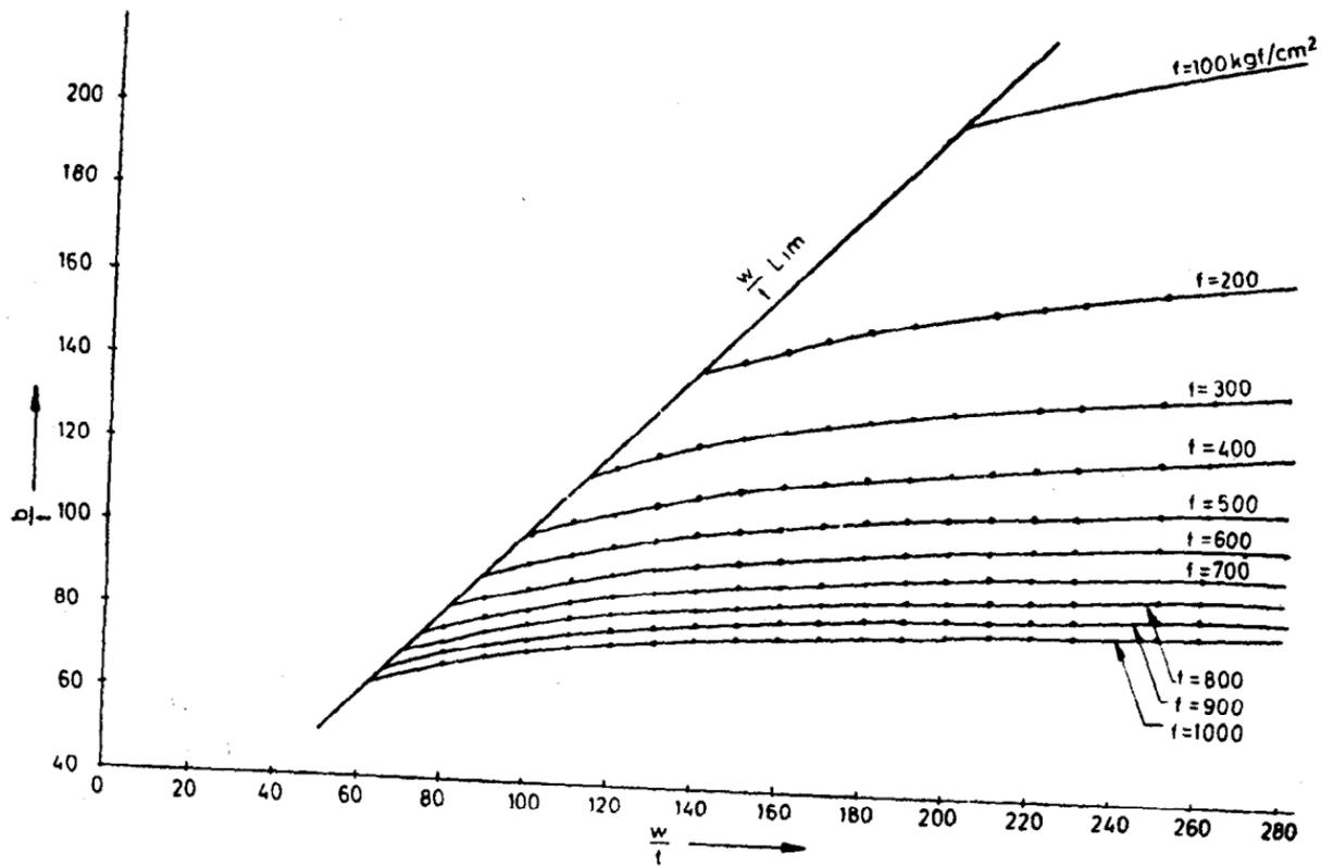
FIG. 28A  $\frac{b}{t}$ -RATIO FOR DEFLECTION DETERMINATION ( TUBULAR SECTIONS )
