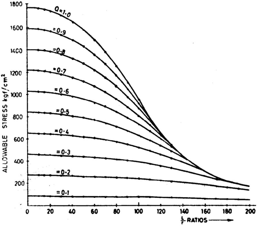
FIG 36 ALLOWABLE COMPRESSIVE STRESS IN kgf/cm<sup>2</sup>,
