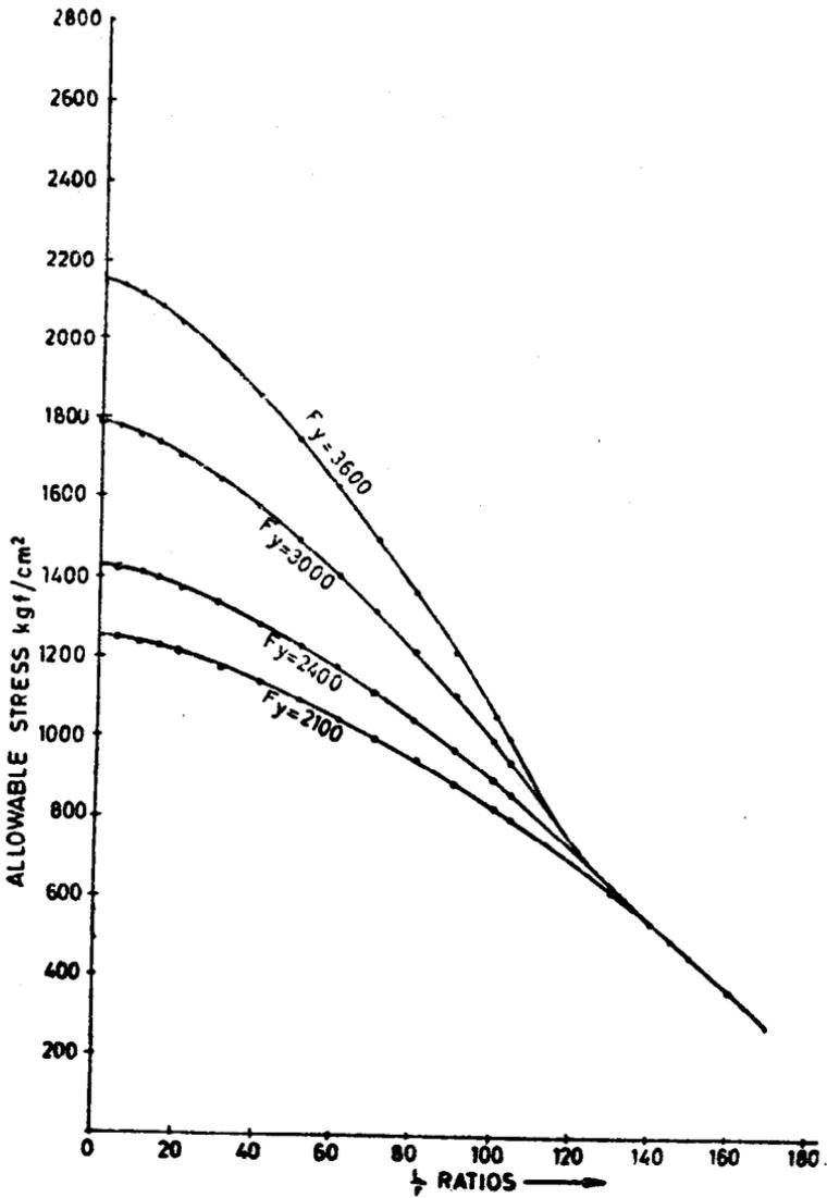
FIG. 37 ALLOWABLE COMPRESSIVE STRESS IN kgf/cm<sup>2</sup>
