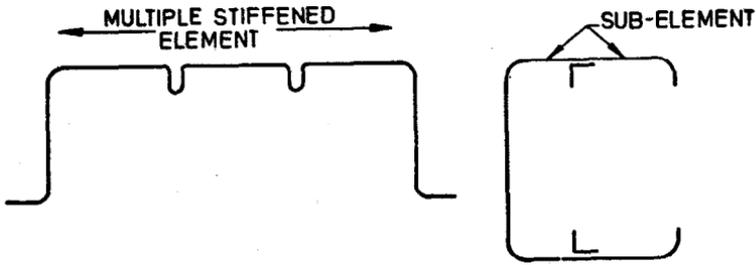
FIG. 5 MULTIPLE STIFFENED ELEMENT AND SUB-ELEMENT
