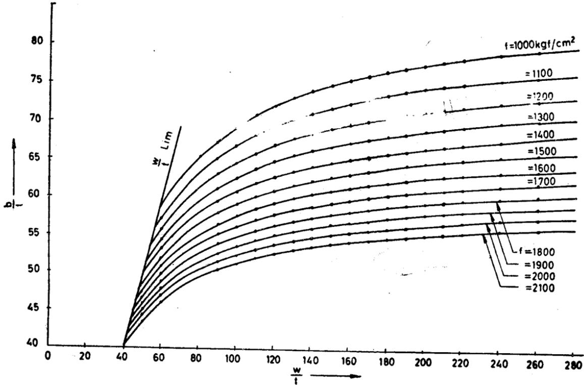
FIG. 26B  $\frac{b}{t}$  RATIO FOR DEFLECTION DETERMINATION (NON-TUBULAR SECTIONS)
