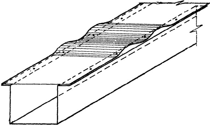
FIG. 24 PLATE SPOT-WELDED TO HAT SECTION
