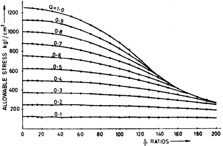
FIG. 34 ALLOWABLE COMPRESSIVE STRESS IN kgf/cm<sup>2</sup>,
