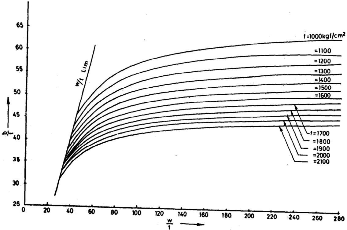
FIG. 25B  $\frac{b}{t}$  RATIO FOR LOAD DETERMINATION (NON-TUBULAR SECTIONS)
