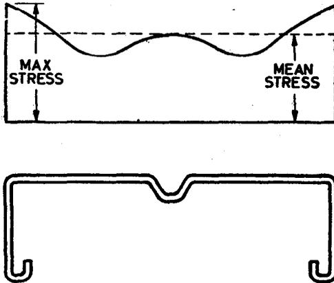
FIG. 14 MULTIPLE STIFFENED ELEMENT
