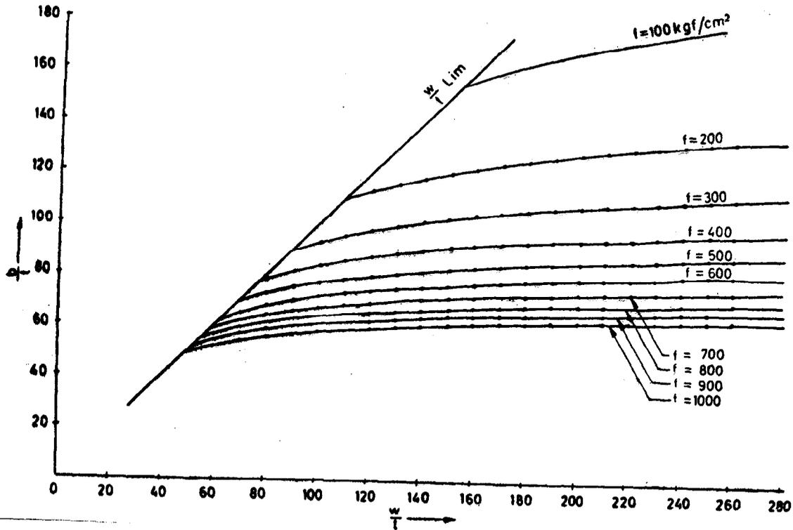
FIG. 27A  $\frac{b}{s}$  RATIO FOR LOAD DETERMINATION ( TUBULAR SECTIONS )
