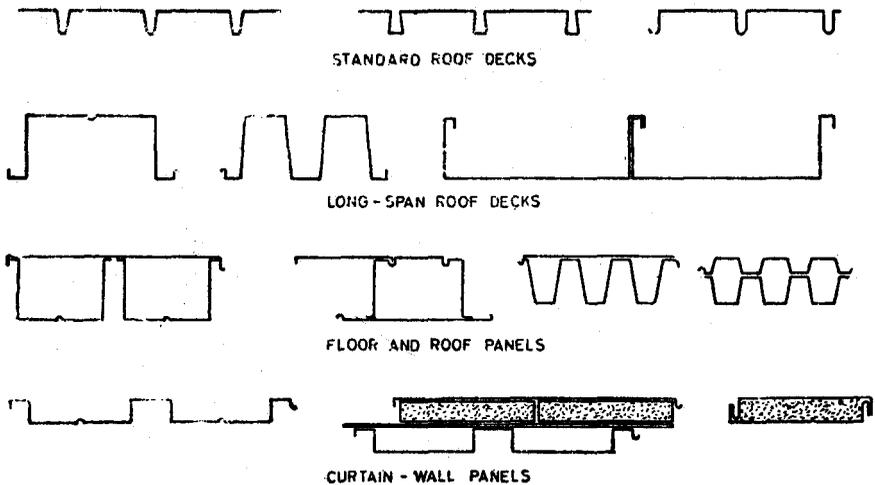
FIG. 2 FLOOR AND ROOF DECKS, AND WALL PANELS
