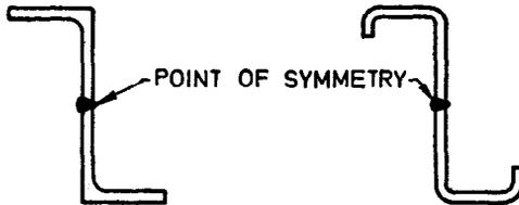
FIG. 9 POINT SYMMETRIC SECTION
