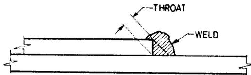
FIG. 23 THROAT OF A FILLET WELD
