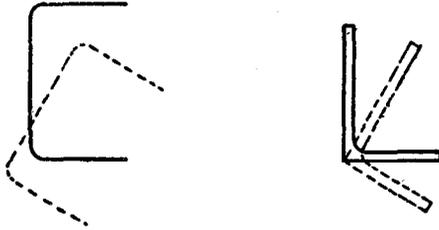
( The cross section shown dotted after buckling )
