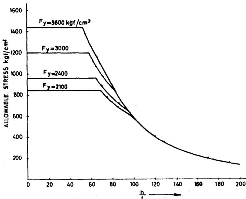
FIG. 32 ALLOWABLE SHEAR STRESS IN WEBS IN kgf/cm<sup>2</sup>
