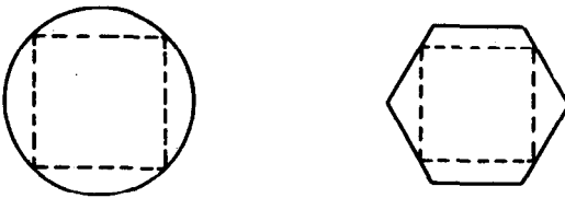
Fig. E-42 Face of the Column for Computing Stresses in Round and Octagonal Columns
