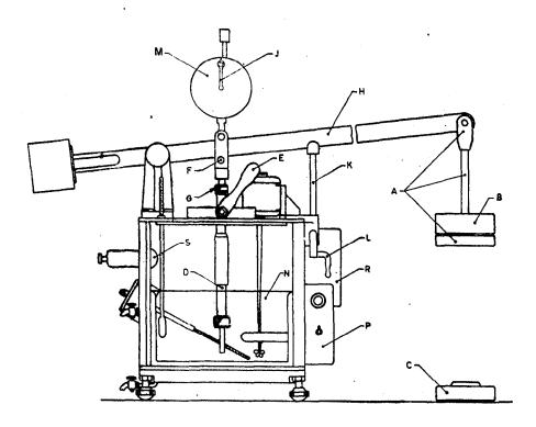
3 - Indicating needle A - Yoke, stalk and tray B — Weight (central hole) K — Beam support yoke C - Weight (slotted) L - Support bracket D - Indentor pin spindle M - Calibrated dial N - Water bath E - Lock lever P - Controls for water stirrer F - Spindle head R — Controls for heater blade and thermostat G - Adjusting nut S - Bath illuminator H - Beam
