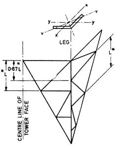
Method of Loading/ Rigidity of Joints
