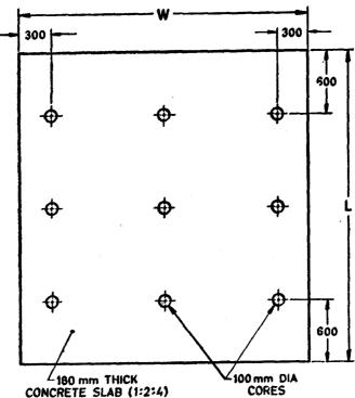
W = Clear width of pavement slab between the forms and should suit the length of vibrating beam (see IS: 2506-1964 'Specification for screed board concrete vibrators')
