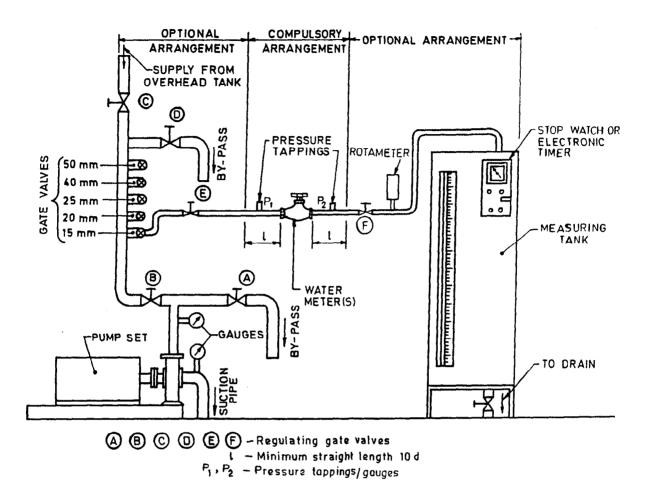
NOTE — By operating the appropriate valves, the set-up can be connected either to the overhead tank or to the pump-set. It is advisable to provide a pressure gauge near the delivery line and a control valve for initial starting of the pump.
