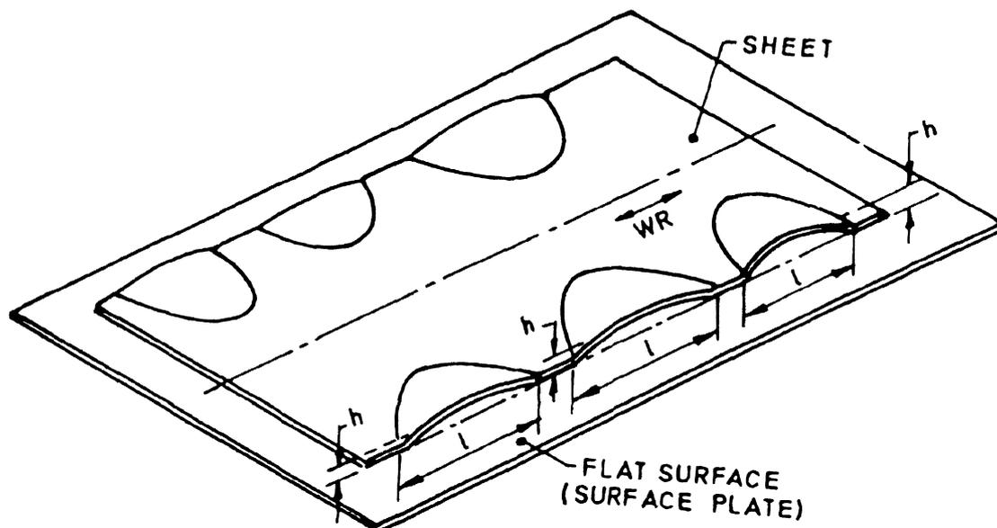
FIG. 17 EXAMPLE OF WAVE FORMATION AT EDGE
