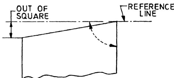
FIG. 13 OUT OF SQUARE TOLERANCE FOR CUT LENGTH
