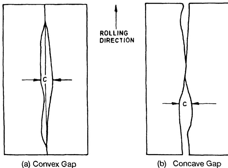
FIG. 11 DEVIATION FROM THE SHEARING LINE DUE TO INTERNAL STRESSES
