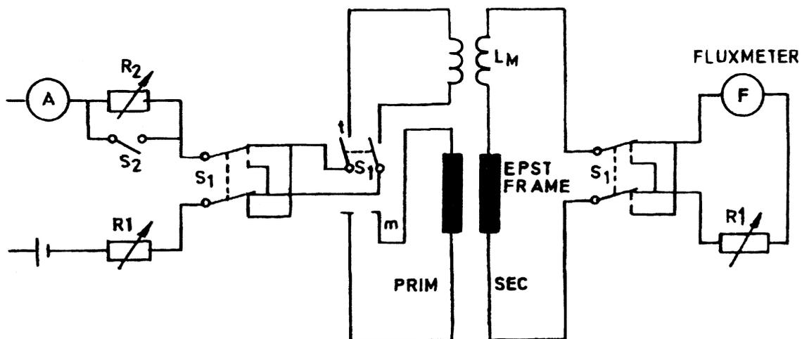
FIG. 5 CIRCUIT FOR D.C. TESTING
