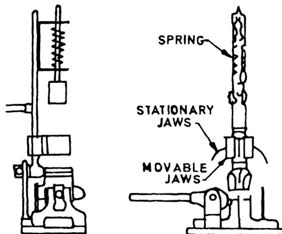
FIG. 9 APPARATUS FOR BEND TEST
