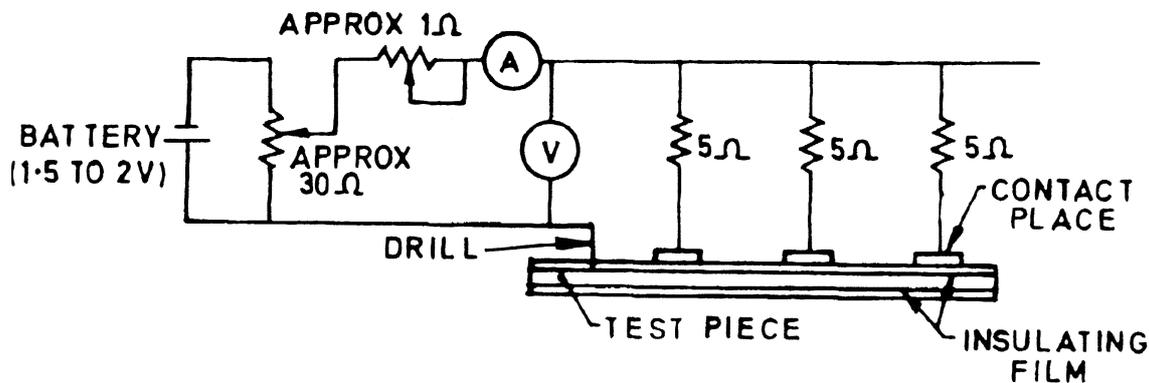
FIG. 7 CONNECTIONS FOR CONTACTS AND RESISTORS
