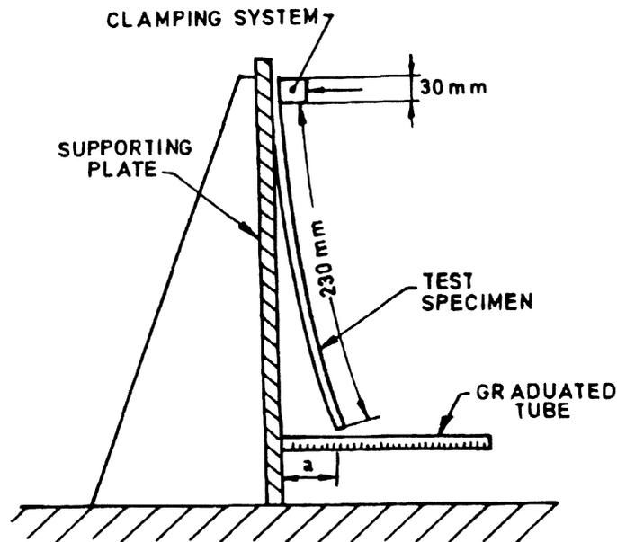
FIG. 18 MEASURING DEVICE FOR BOWING
