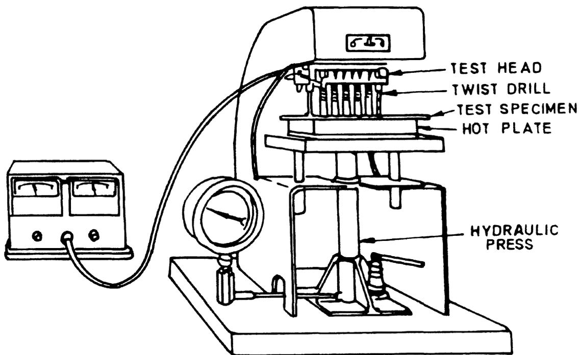
FIG. 6 APPARATUS OF SURFACE INSULATION RESISTIVITY MEASUREMENT
