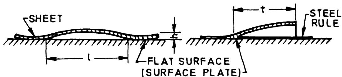
FIG. 16 CHARACTERISTIC VALUES FOR THE DETERMINATION OF WAVINESS
