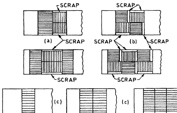
FIG. 1 SUGGESTED DISTRIBUTION OF STRIP TO BE CUT FROM SHEETS FOR MAGNETIC TESTS
