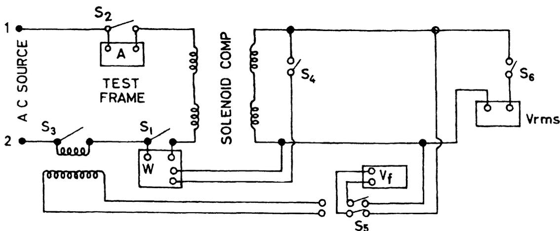
FIG. 2 BASIC CIRCUIT DIAGRAM FOR WATTMETER METHOD
