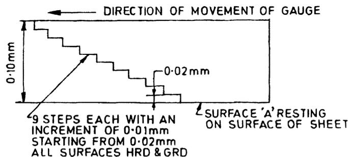
FIG. 15 STEPPED CHECKING GAUGE FOR BURR ON EDGE
