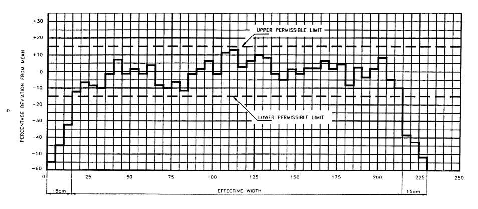
Fig. 1 Typical Results of Test for Uniformity of Transverse Distribution of Binder
