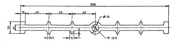
All dimensions in millimetres. FIG. 1 TYPICAL CROSS-SECTION OF PVC WATER-STOP
