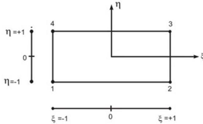
**Fig. 3.4.4 Four node rectangular element**
