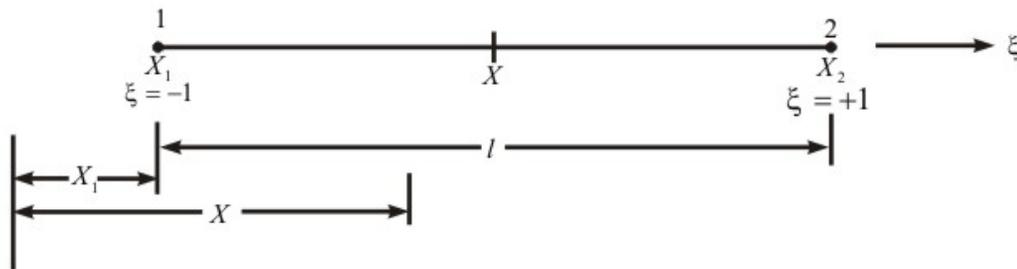
Fig. 3.4.1 Natural coordinates of bar element
