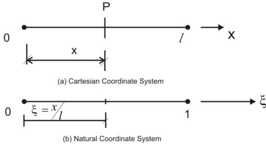
**Fig. 3.1.1 Two node line element**
