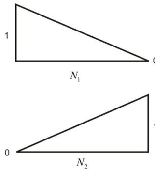
**Fig. 3.1.2 Linear interpolation function for two node line element**
