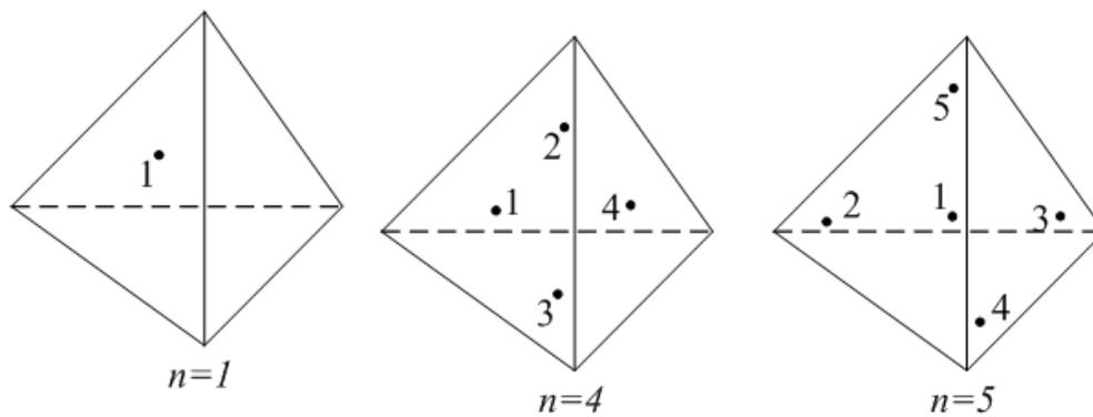
**Fig. 3.9.3 Gauss points for tetrahedrons**
