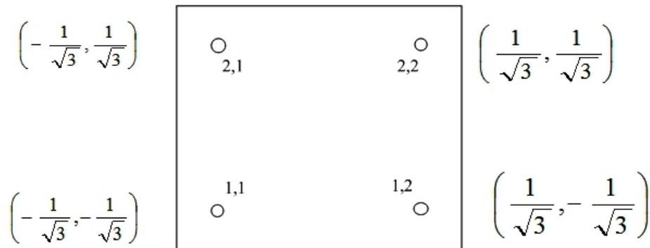
**Fig. 3.9.1 Gauss points for two-dimensional integral**
