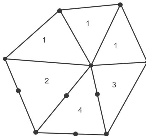
**Fig. 3.2.5 Triangular elements with different number of nodes**
