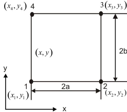
**Fig. 3.3.2 Rectangular element in Cartesian coordinate**
