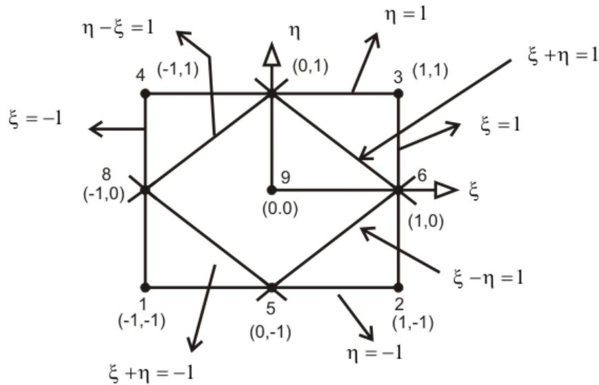
**Fig. 3.4.9 Equations of lines for two dimensional eight node element**
