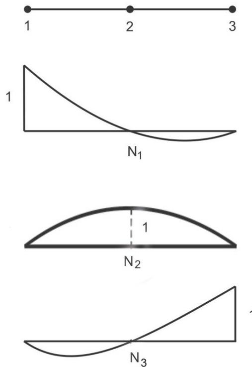
**Fig. 3.1.3 Variation of interpolation function for three node line element**
