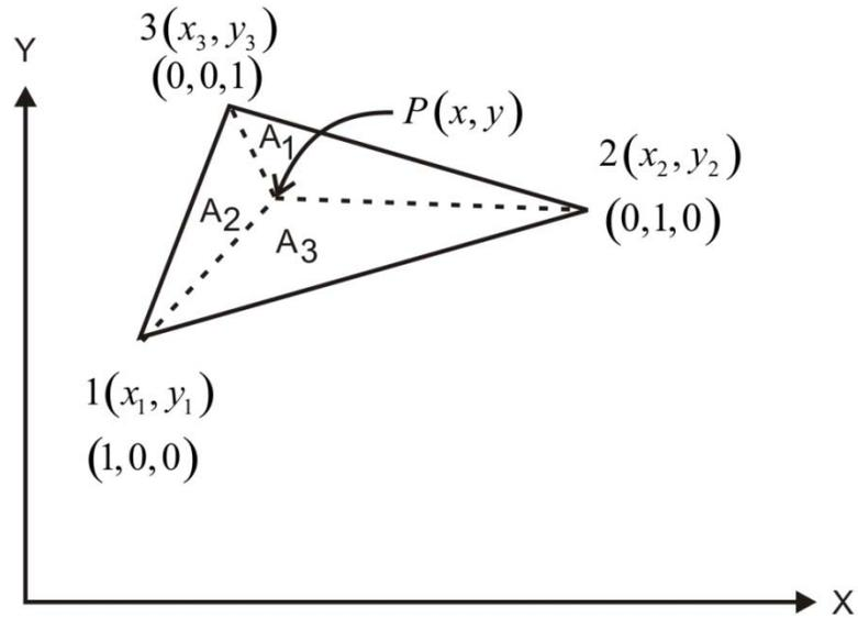
**Fig. 3.1.4 Triangular coordinate system**
