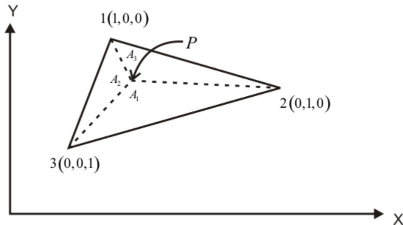
**Fig. 3.1.5 Area coordinates for triangular element**
