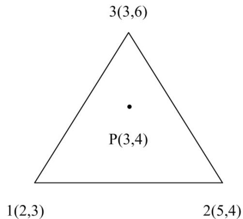
**Fig. Ex.3.1 Nodal coordinates of a triangular element**
