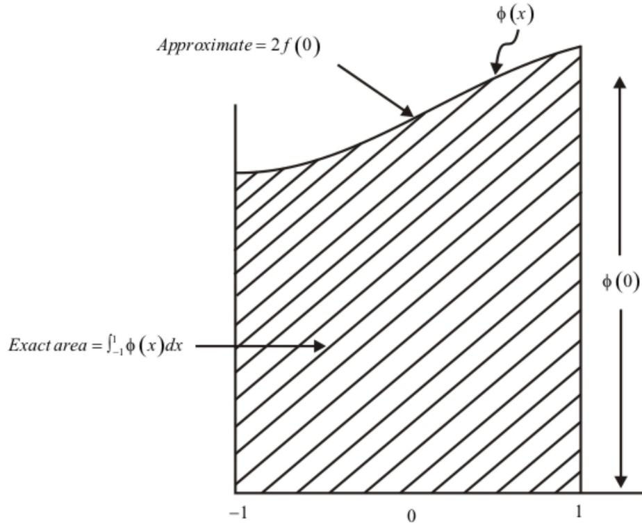
**Fig 3.8.1 One-point Gauss Quadrature**
