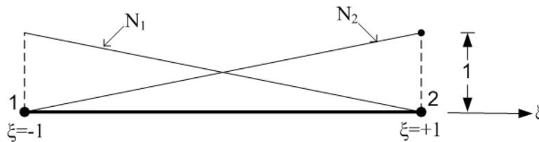
**Fig. 3.4.2 Shape functions for two node bar element**
