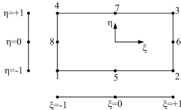
**Fig. 3.3.4 Natural coordinates of eight node rectangular element**
