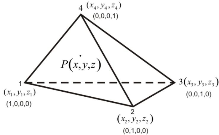
**Fig. 3.5.3 Four node tetrahedron element**
