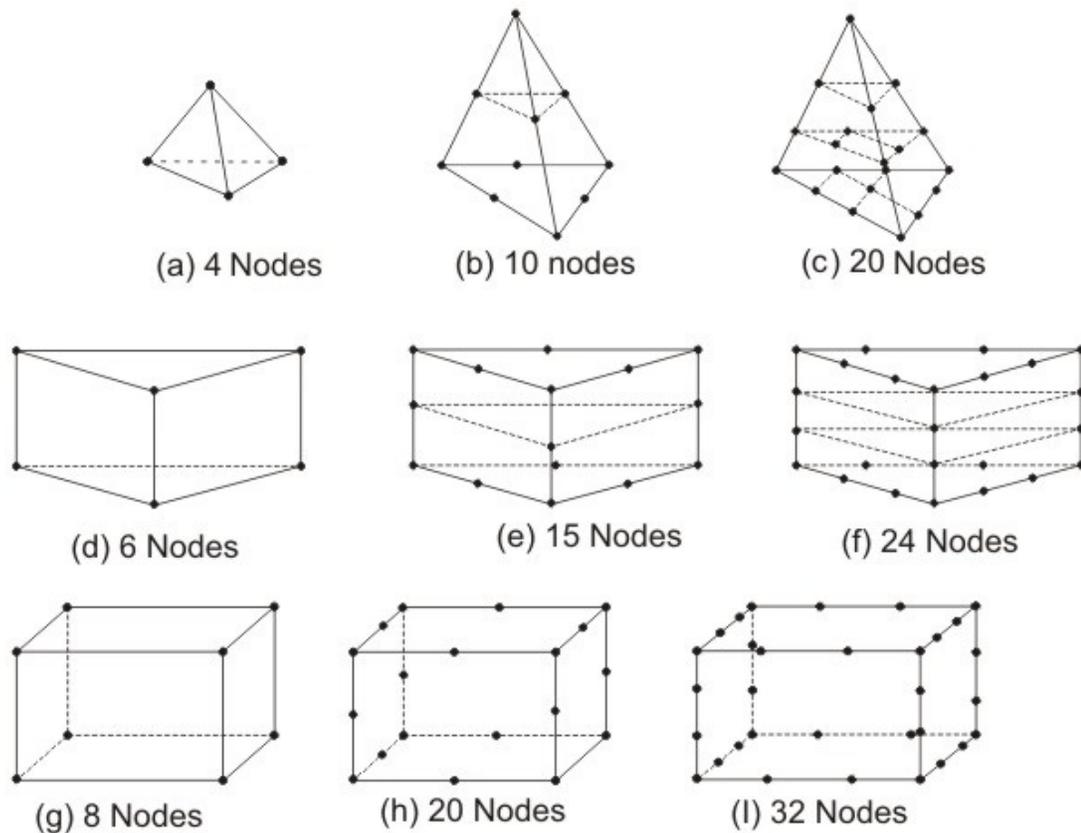
**Fig. 3.5.1 Three-dimensional solid elements**
