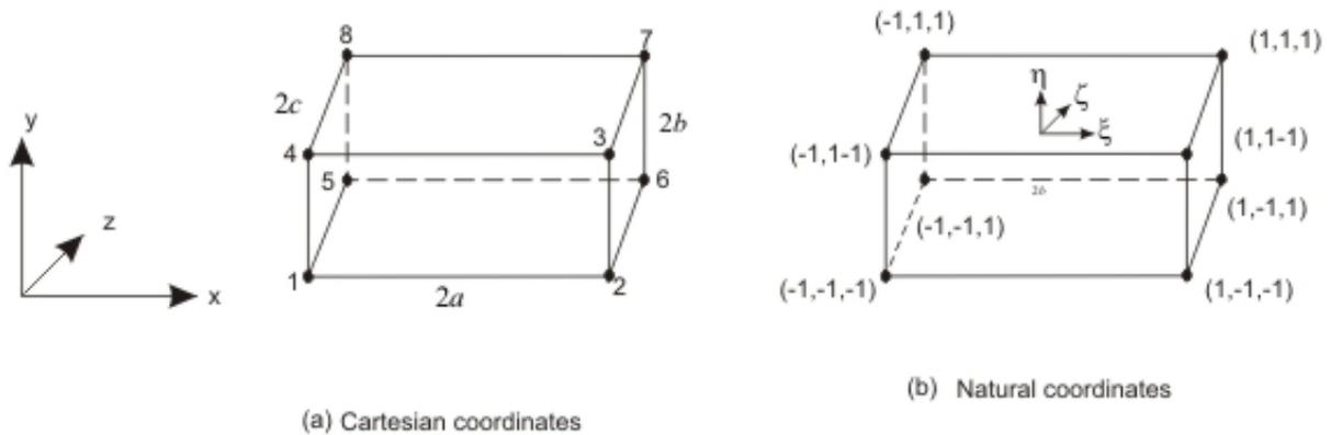
**Fig. 3.5.4 Eight node brick element**
