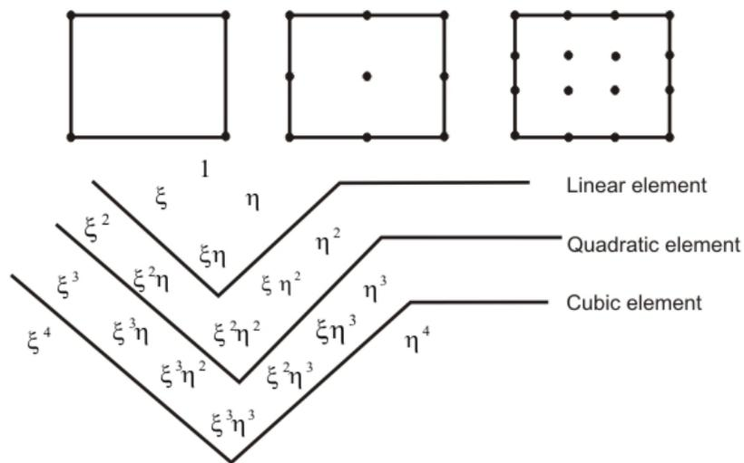
**Fig. 3.4.6 Two dimensional Lagrange elements and Pascal triangle**
