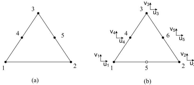
**Fig. 3.2.6 Degrading for five node element**
