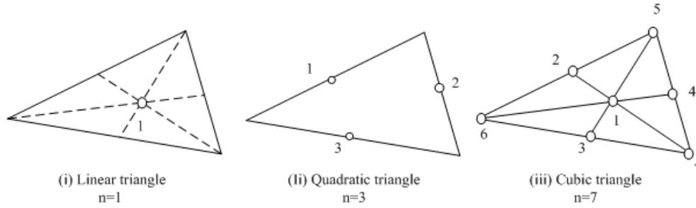
**Fig. 3.9.2 Gauss points for triangles**
