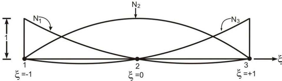
**Fig. 3.4.3 Quadratic shape functions for three node bar element**
