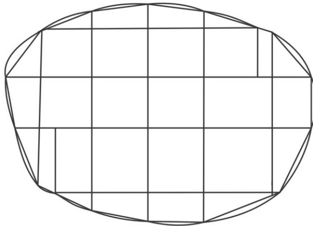
**Fig. 3.2.1** Finite element mesh consisting of triangular and rectangular element
