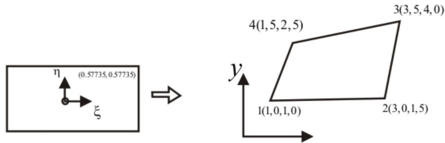
**Fig. 3.7.1 Two dimensional quadrilateral element**
