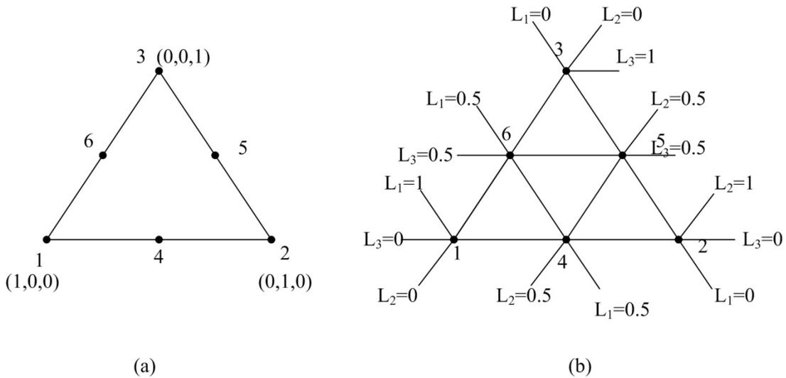
**Fig. 3.2.4 (a) Six node triangular element (b) Lines of constant values of the area coordinates**
