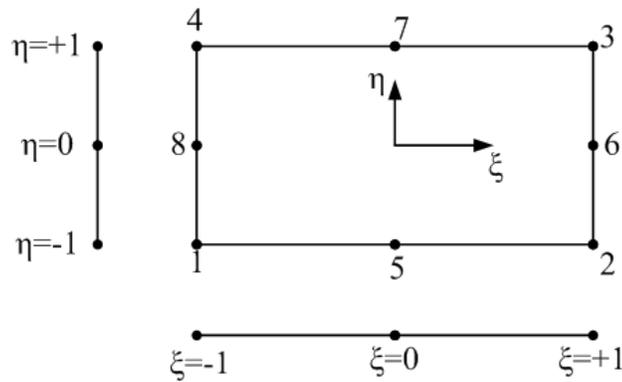
**Fig. 3.4.8 Two dimensional eight node rectangular element**
