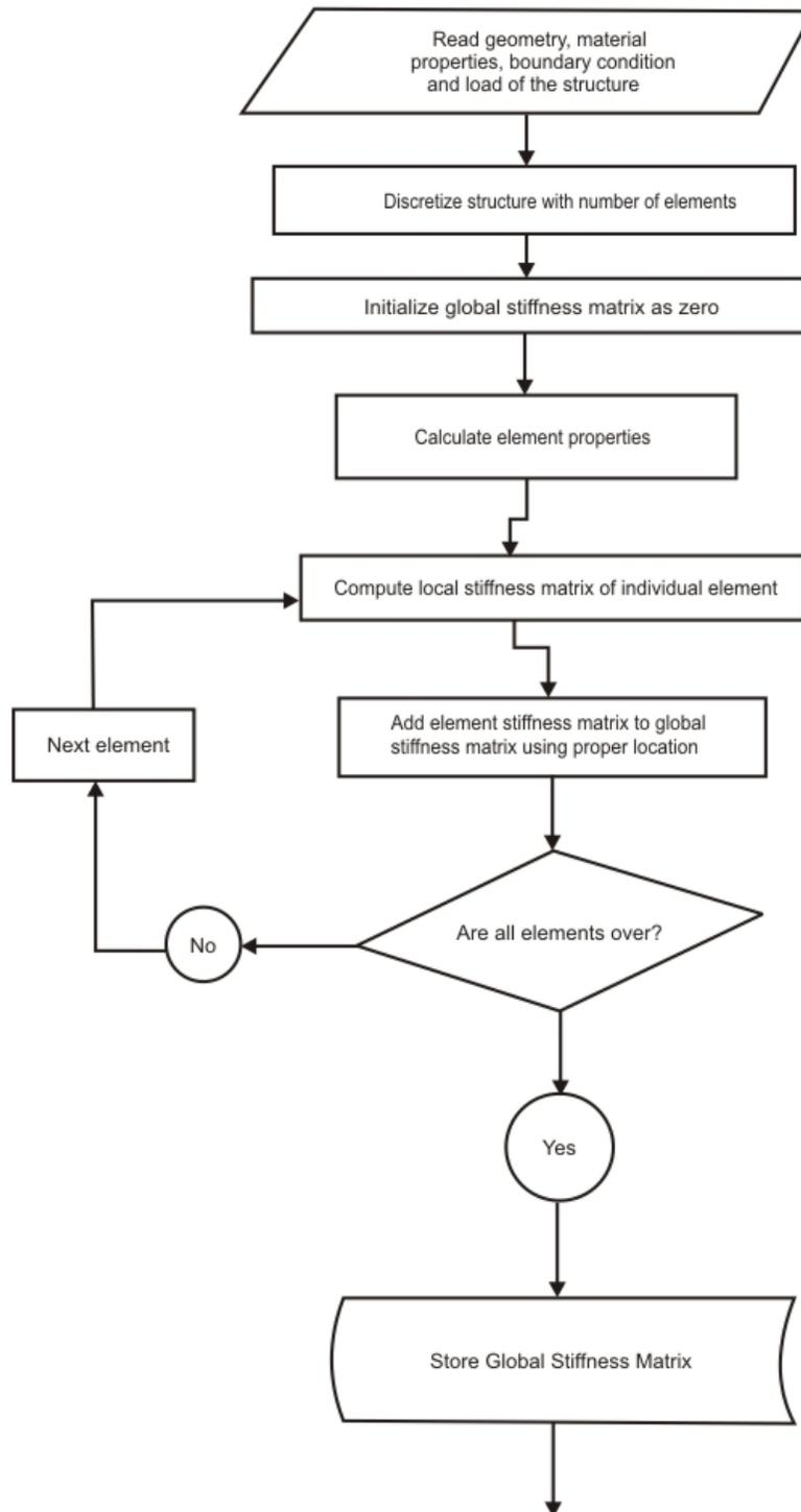
**Fig. 2.4.1** Assemble of stiffness matrix from local to global
