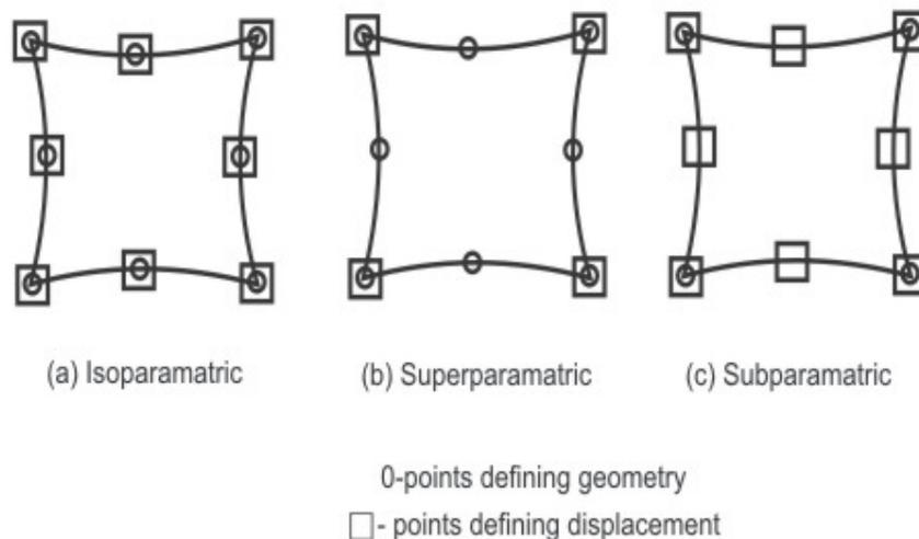
**Fig. 2.3.2 Shape functions for geometry and displacements**
