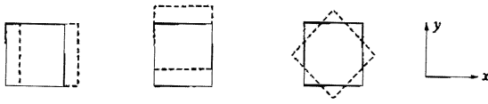
(a) Rigid-body modes of a plane stress element (from left to right, pure translation in x and y directions and pure rotation)
