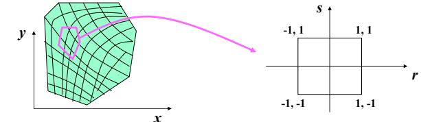
In general we would like to be able to represent any element in a standardized manner – introducing a transformation between the natural coordinates and the real coordinates (global)
