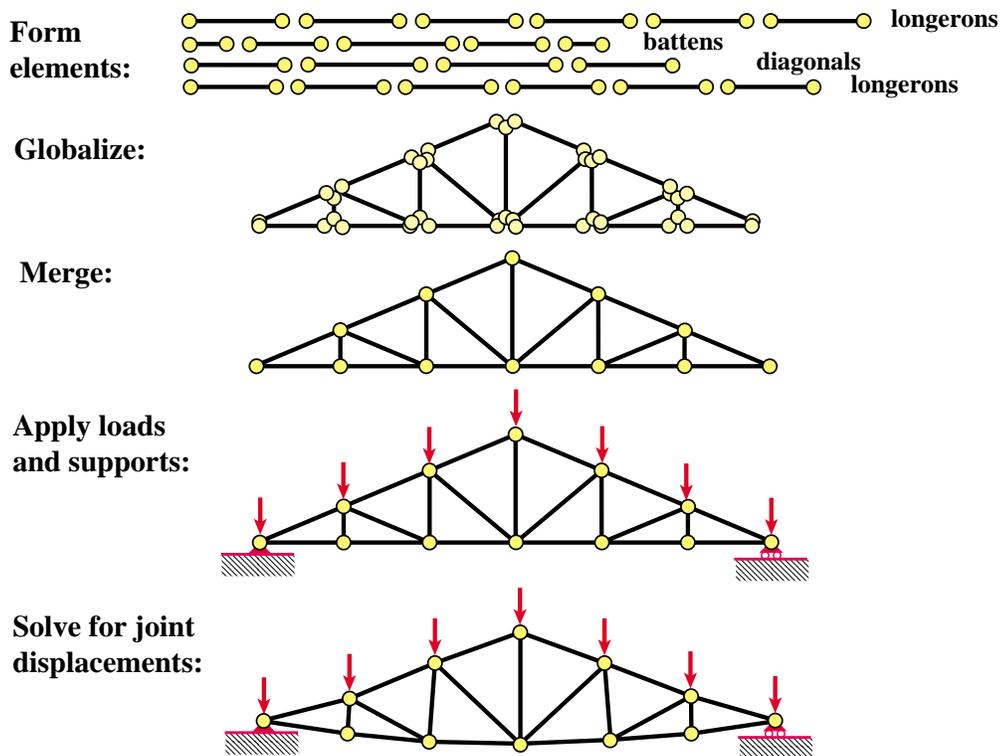
FIGURE 2.7. Visualization of the DSM assembly-and-solution stage.
