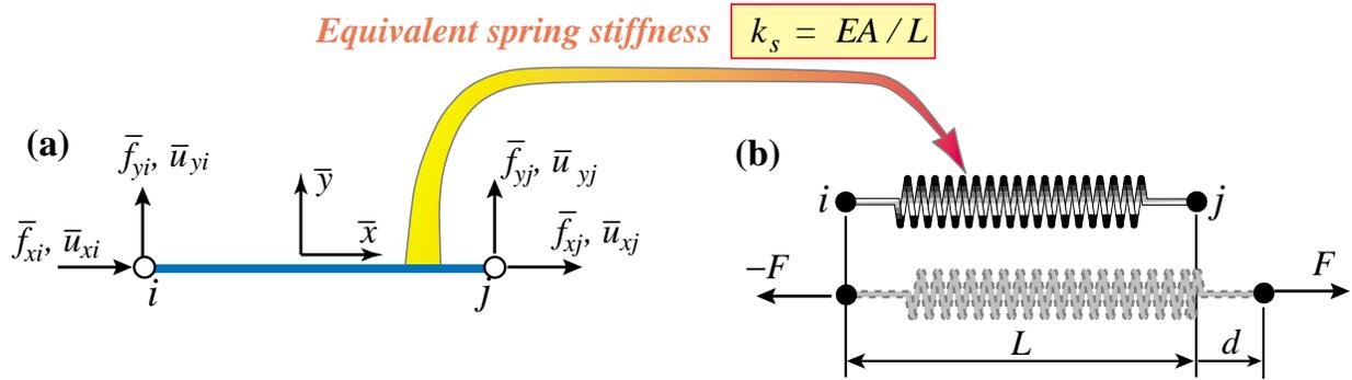
FIGURE 2.9. Generic truss member referred to its local coordinate system  $\{\bar{x}, \bar{y}\}$ : (a) idealization as 2-node bar element, (b) interpretation as equivalent spring. Element identification number  $e$  dropped to reduce clutter.
