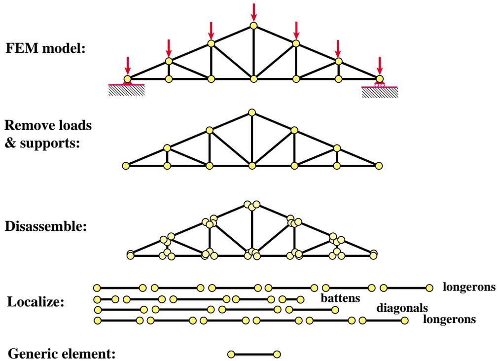
FIGURE 2.6. Visualization of the DSM breakdown stage.
