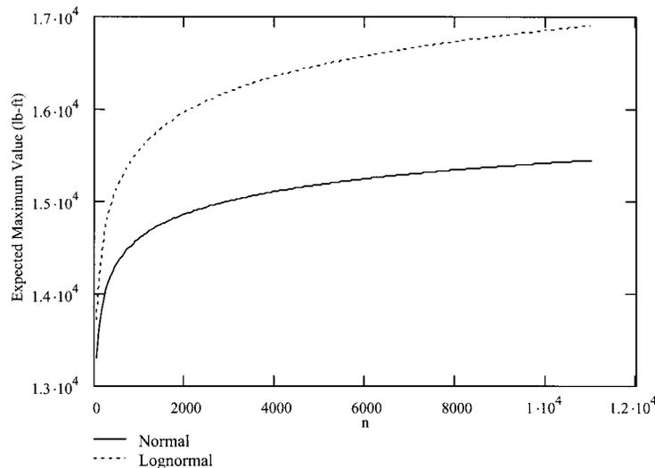
FIG. 7. Mean Maximum Midspan Bending Moment As Function of Number of Realizations (1 lb/ft = 1.26 N/m)
