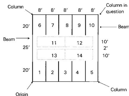
FIG. 10. Vehicle and Stall Layout for 10-Stall Bay (1 ft = 0.3048 m)
