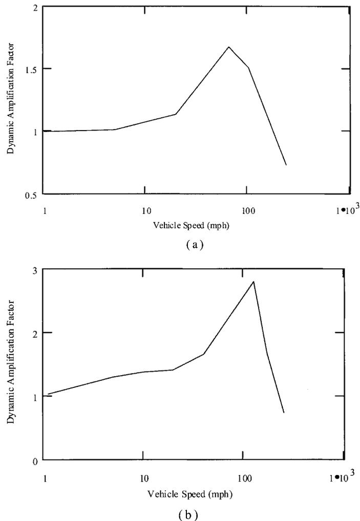
FIG. 9. Dynamic Amplification Factor As Function of Vehicle Speed: (a) Simply Supported Slab; (b) Clamped Slab (1 mph = 1.6 km/h)
