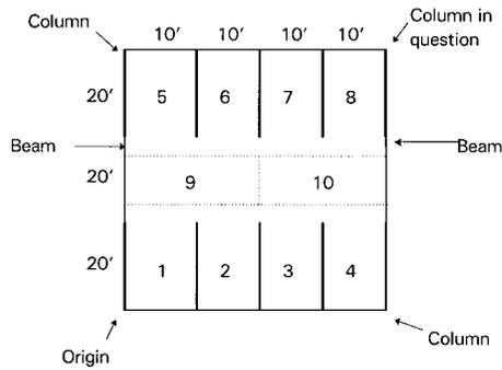
FIG. 3. Stall Layout and Vehicle Position for Evaluation of Column Axial Force and Midspan Beam Moment (1 ft = 0.3048 m)
