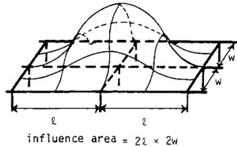
FIG. 4. Influence Surface for Column Axial Loading
