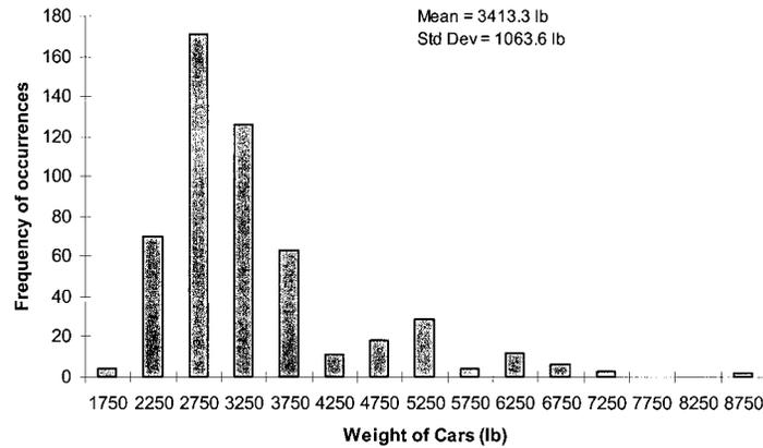
FIG. 1. Histogram of Parking Garage Vehicle Weights (1 lb = 0.454 kg)
