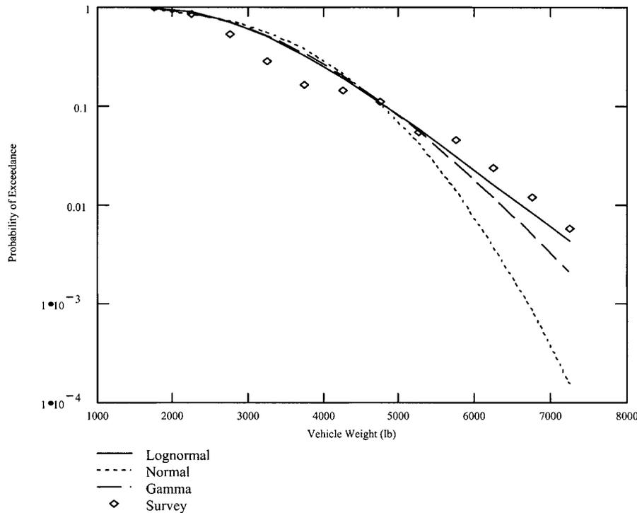
FIG. 2. Probability Distribution of Parking Garage Vehicle Weights (1 lb = 0.454 kg)
