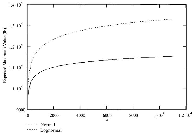
FIG. 5. Mean Maximum Column Axial Force As Function of Number of Realizations (1 lb = 0.454 kg)
