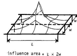
FIG. 6. Influence Surface for Beam Midspan Moment
