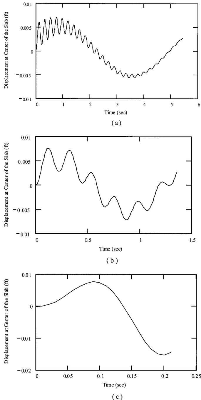
FIG. 8. Displacement at Center of Slab for: (a)  $V = 8$  km/h (5 mph); (b)  $V = 32$  km/h (20 mph); (c)  $V = 202$  km/h (126 mph) (1 ft = 0.3048 m)
