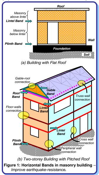
flat timber or CGI sheet roof, roof band needs to be provided. In buildings with pitched or sloped roof, the roof band is very important. Plinth bands are primarily used when there is concern about uneven settlement of foundation soil.
